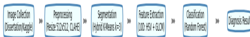
Figure 1: Flow of the diagram of the proposed pipeline for sugarcane disease identification
