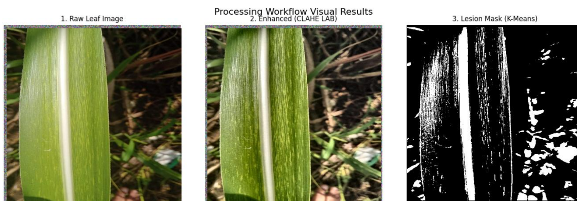
Figure 4: Visual Outcomes of the Image Processing Workflow for Leaf Lesion Detection.
